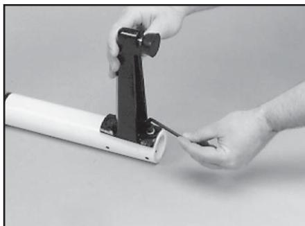
Align the holes in the leg flange with the matching holes in the lower column support post. Secure the leg with one FLAT HEAD cap screw through the upper hole, and one SOCKET HEAD cap screw through the bottom hole. Repeat this procedure for the three remaining legs.
