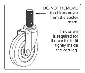
Step 1: Insert caster into the bottom of the cart leg.
